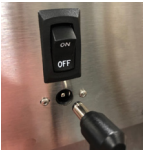
Inlet supply connector being plugged in
