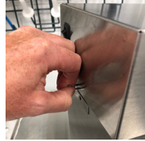
Pulling locking spring pin out to unlock the back of the lid
